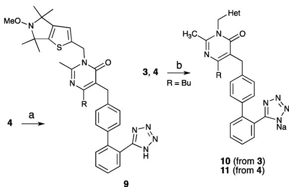
**Scheme 2** Reagents and conditions: (a) FeSO<sub>4</sub>, DMSO, H<sub>2</sub>O<sub>2</sub>, 89%; (b) NaH, THF, 85%.
