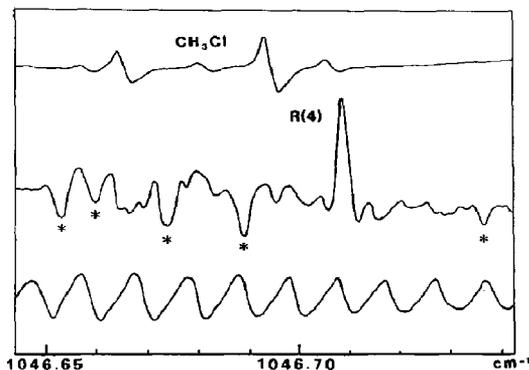
Fig. 2. Observed spectrum for the R(4) line of the  $\text{SiF}^+$  ion. The  $\text{SiF}_4$  lines (asterisked) are observed with signs opposite to that for the ion line. The spectrum of  $\text{CH}_3\text{Cl}$  (top) and the etalon fringe (bottom) were used for the wavenumber calibration.
