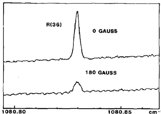
Fig. 3. Magnetic field effect on the R(36) line of  $\text{SiF}^+$ . The spectrum was observed by discharge modulation with 800 mA p-p current.
