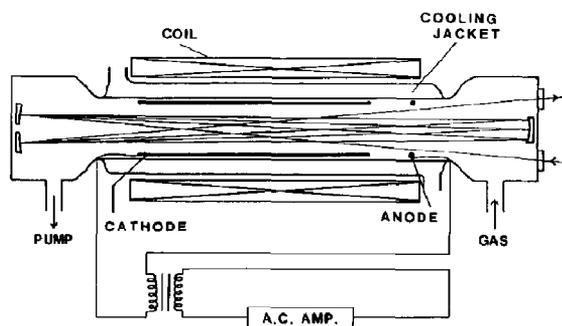
Fig. 1. Schematic diagram of the hollow cathode discharge cell. A 3 kHz ac high voltage stepped up by a transformer is applied between the electrodes to produce a glow discharge. The three concave mirrors form a White-type multireflection optical path. The solenoid coil is used to check the magnetic field effect on the ion lines.
