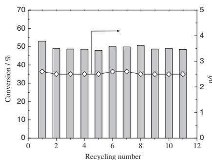
**Figure 1.** The recycling results of 1-hexene hydroformylation over catalysts TMGL–TPPTS–Rh/MCM-41. TMGL loading = 10 wt %, Rh loading = 0.8 wt % based on silicas, TPPTS/Rh = 5 (molar ratio).
