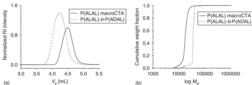
**Fig. 1.** (a) RI traces and (b) cumulative weight fractions for the P(ALAL) macroCTA ( $M_n$  16900 g mol<sup>-1</sup>, PDI 1.09) and P(ALAL)-*b*-P(ADAL) ( $M_n$  33900 g mol<sup>-1</sup>, PDI 1.04).
