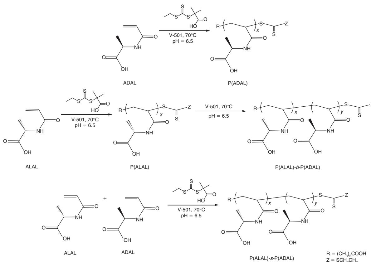
**Scheme 1.** Pathway for aqueous RAFT synthesis of acryloyl-D- and L-alanine homopolymers, block copolymers, and a statistical copolymer.
