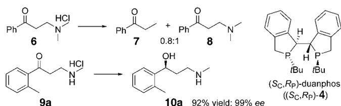
**Scheme 2.** Asymmetric hydrogenation of  $\beta$ -amino ketone hydrochlorides with  $[\text{Rh}\{(\text{S}_C, \text{R}_P)\text{-4}\}(\text{nbd})\text{SbF}_6$  (**5a**) as the catalyst. Reaction conditions: **5a** (0.5 mol%), MeOH,  $\text{K}_2\text{CO}_3$  (0.5 equiv),  $\text{H}_2$  (10 bar),  $50^\circ\text{C}$ , 12 h. nbd = norbornadiene.
