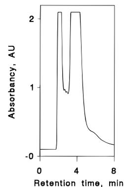
Figure 7. Enantioseparation of racemic 3,5-dinitrobenzamidoleucine-*N,N*-diallylamide (**Ia**) on chiral stationary phase CSP 2 under overload conditions. Conditions: column size, 150 mm  $\times$  4.6 mm i.d.; mobile phase, 20% hexane in dichloromethane; flow rate, 1 mL/min; injection, 0.5 mg.
