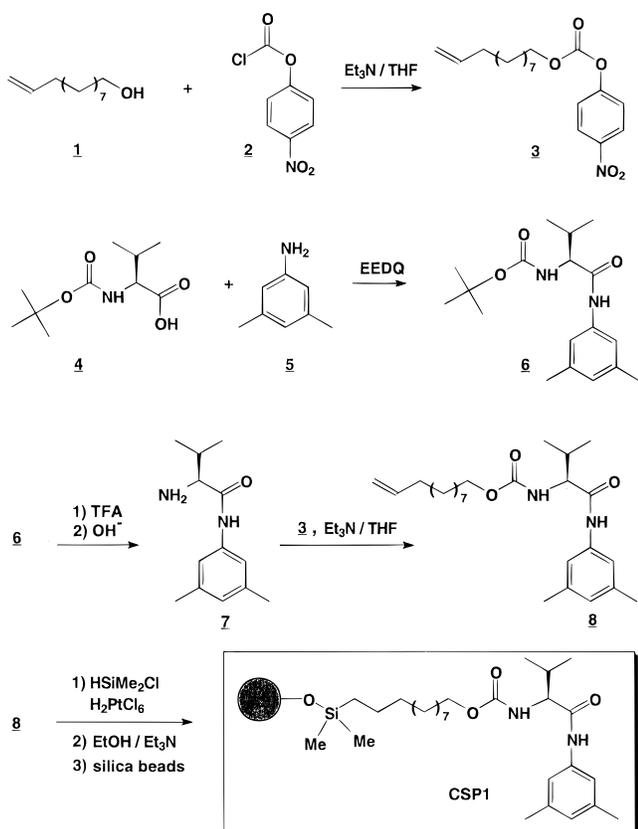
Figure 4. Synthetic strategy for the preparation of the silica-based chiral stationary phase (CSP 1).
