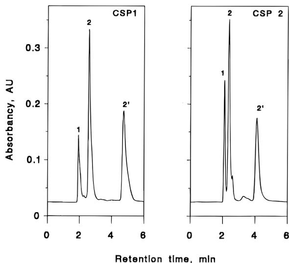
Figure 6. Separation of 3,5-dinitrobenzamidoleucine-*N,N*-diallylamide (**Ia**) enantiomers on chiral stationary phases CSP 1 and CSP 2. Conditions: column size, 150 mm  $\times$  4.6 mm i.d.; mobile phase, 20% hexane in dichloromethane; flow rate, 1 mL/min; injection, 7  $\mu$ g; peaks, 1,3,5-tri-*tert*-butylbenzene (1), *R*-enantiomer (2), *S*-enantiomer (2').
