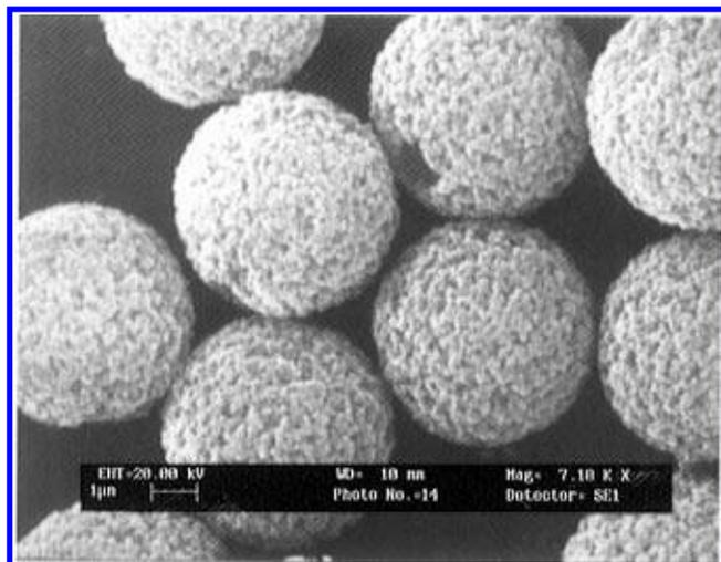
Figure 3. Scanning electron micrograph of the monodispersed macroporous poly(glycidyl methacrylate-co-ethylene dimethacrylate) beads.
