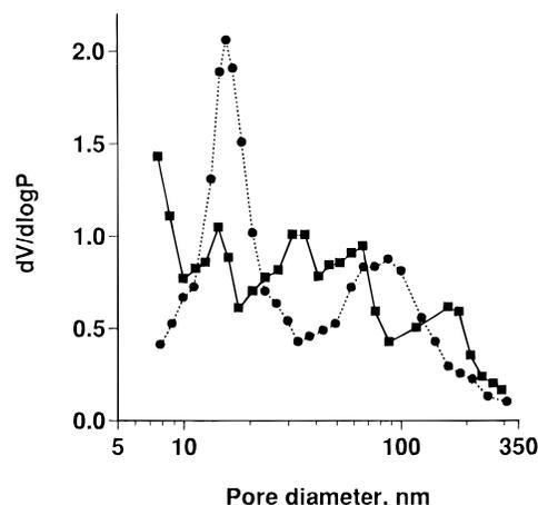
Figure 2. Differential pore size distribution curves for the silica beads (dotted line) and the monodisperse polymer beads (solid line) as determined by mercury intrusion porosimetry.
