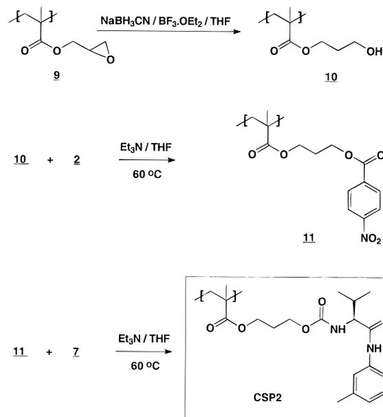
Figure 5. Synthetic strategy for the preparation of the polymer-based chiral stationary phase (CSP 2).
