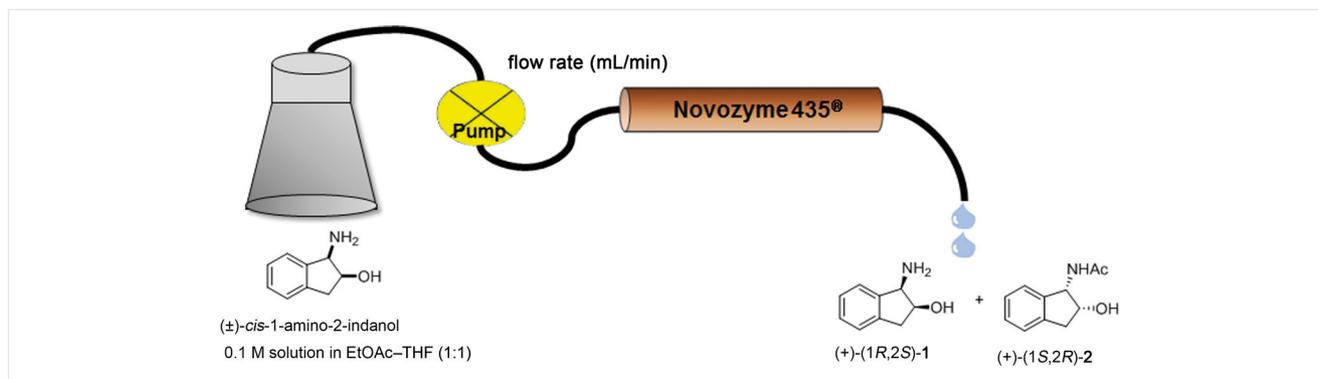
**Figure 1** Schematic diagram of the continuous-flow system for kinetic resolution of ( $\pm$ )-*cis*-1-amino-2-indanol
