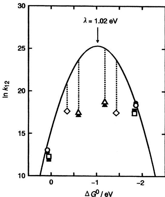
Fig. 3. Driving force dependence of the rate constants for the quenching and back ET reactions of ZnMb with quinolinium ions and viologens. (○) **2a**, (●) **2b**, (□) **3a**, (■) **3b**, (△) (*S,S*)-OAV<sup>2+</sup>, (▲) (*R,R*)-OAV<sup>2+</sup>, and (◇) MV<sup>2+</sup>. The solid curve is calculated by Eq. 4 with  $\lambda_{12} = 1.02$  eV.
