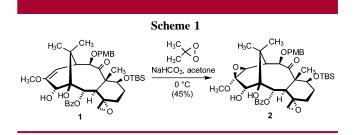
under dilute reaction conditions. The acquisition of HMBS, COSY, and HMQC data convincingly established the product to be the C12–C13 oxirane having an exo-oriented heteroatom.
