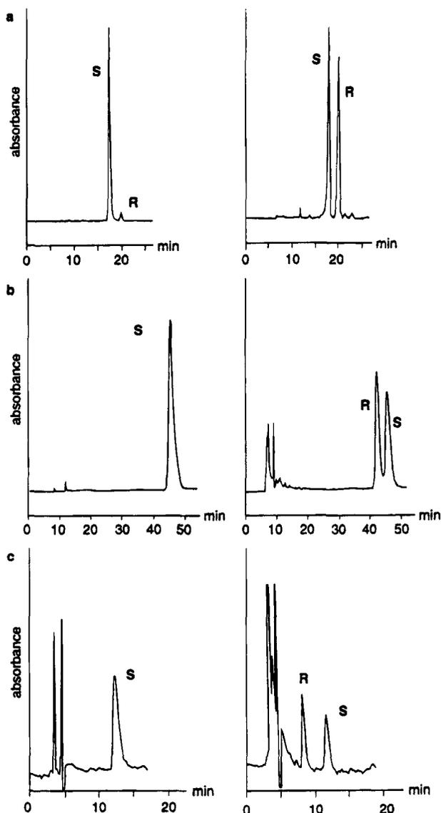
**Figure 2.** Enantiopurities of (a) **2a**, (b) **2d**, and (c) **2f** determined by HPLC on a chiral stationary phase and compared with the corresponding racemates (right). See Table 1 and ref 36 for the experimental conditions.
