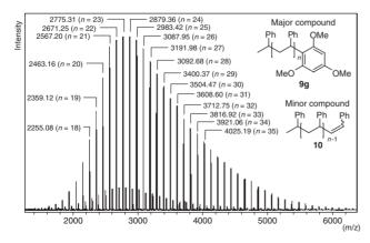
Figure 1. MALDI-TOF mass spectrum of polystyrene 9g and 10 (=93:7). A series of peaks, as indicated by the average mass number, was observed in the silver ion added form  $(M + Ag)^+$ .
