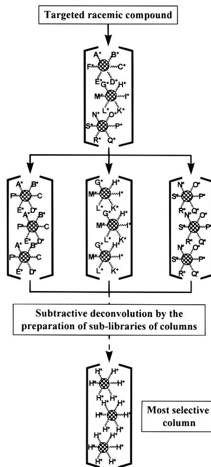
Figure 1. Illustration of the concept applied in an on-bead combinatorial deconvolution scheme to identify an effective selector H\* from a multicompound chiral stationary phase (selector library A\*–S\*).
