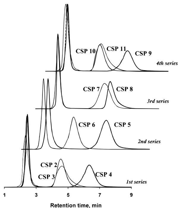
Figure 3. Overlay of chromatograms obtained with CSPs 2–11 prepared in four deconvolution series. Conditions: analyte, (3,5-dinitrobenzoyl)leucine diallylamide; column, 150 × 4.6 mm i.d.; mobile phase, 20% hexane in dichloromethane; flow rate, 1 mL/min, UV detection 254 nm.
