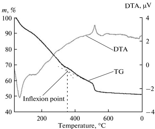
**Fig. 2.** TG-DTA curves for the precursor  $\text{MnCO}_3$ .
