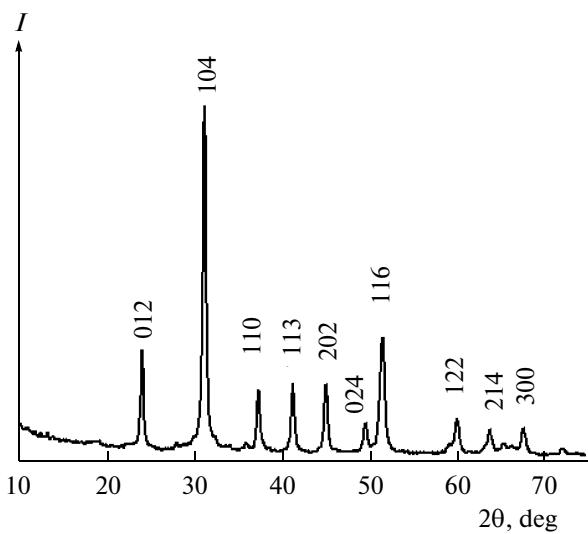
**Fig. 1.** XRD pattern of the precursor  $\text{MnCO}_3$ .
