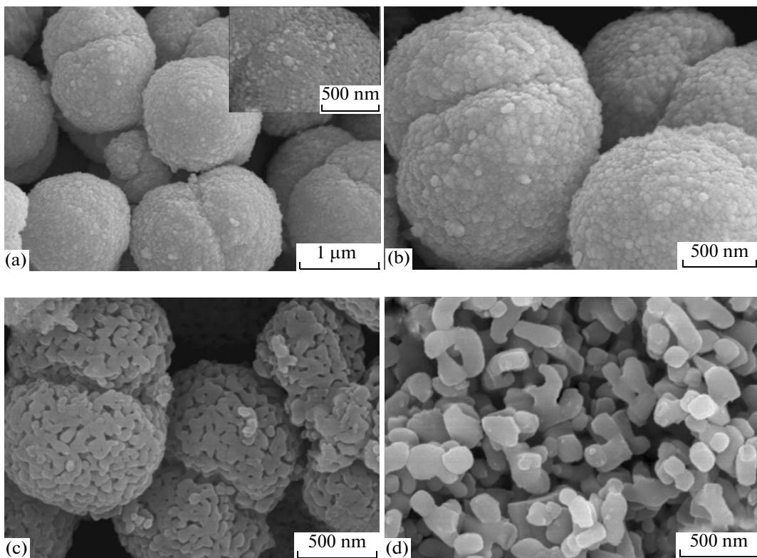
**Fig. 4.** SEM images of the precursor (a), sample CT400 (b), sample CT600 (c), sample CT800 (d).
