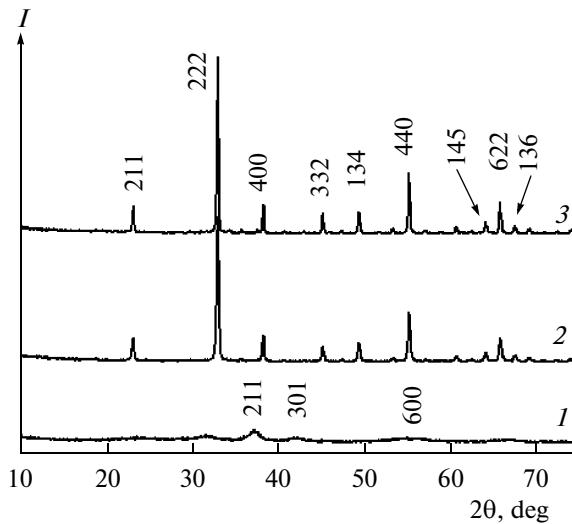
**Fig. 3.** XRD patterns of the calcined samples: CT400 (1), CT600 (2), CT800 (3).
