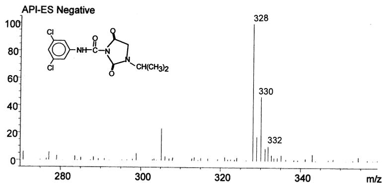
Fig. 8. Mass spectrum of Isomer. Operative conditions are reported in Table 3.
