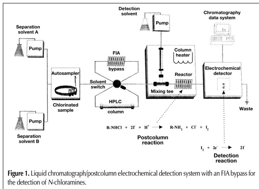
Figure 1. Liquid chromatograph/postcolumn electrochemical detection system with an FIA bypass for the detection of *N*-chloramines.
