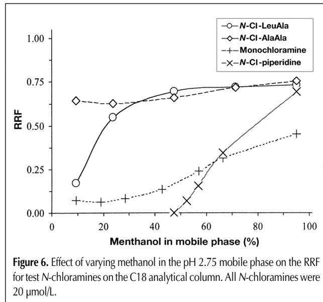
**Figure 6.** Effect of varying methanol in the pH 2.75 mobile phase on the RRF for test *N*-chloramines on the C18 analytical column. All *N*-chloramines were 20  $\mu\text{mol/L}$ .
