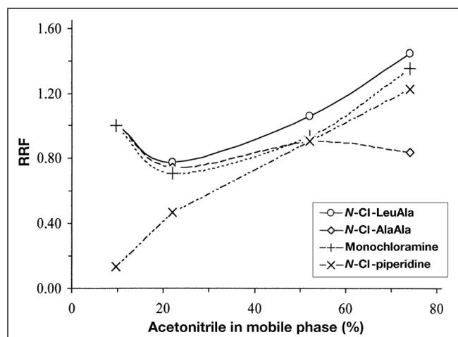
**Figure 7.** Effect of varying acetonitrile in the pH 7.02 mobile phase on the RRF for test *N*-chloramines in a chromatography experiment with the C18 analytical column. All *N*-chloramines were 20  $\mu\text{mol/L}$ .
