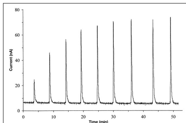
**Figure 9.** Chromatogram of successive monochloramine injections after the C18 column was left overnight with a mostly aqueous mobile phase.
