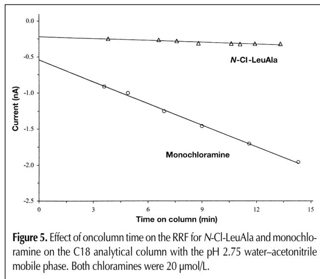
**Figure 5.** Effect of oncolumn time on the RRF for *N*-Cl-LeuAla and monochloramine on the C18 analytical column with the pH 2.75 water-acetonitrile mobile phase. Both chloramines were 20  $\mu\text{mol/L}$ .
