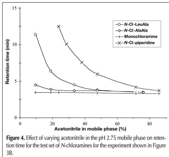
**Figure 4.** Effect of varying acetonitrile in the pH 2.75 mobile phase on retention time for the test set of *N*-chloramines for the experiment shown in Figure 3B.
