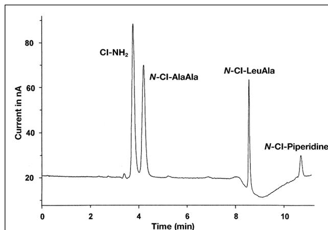
**Figure 10.** Separation of the four test *N*-chloramines using the optimized conditions. The sample was prepared by mixing an equivalent amount of each of the *N*-chloramines, individually prepared as 250- $\mu\text{mol/L}$  amine with 20- $\mu\text{mol/L}$   $\text{OCl}^-$  added, using a 0.5- $\text{mmol/L}$  phosphate buffer (pH 7).
