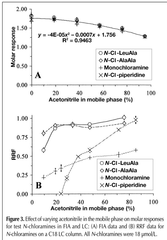
**Figure 3.** Effect of varying acetonitrile in the mobile phase on molar responses for test *N*-chloramines in FIA and LC: (A) FIA data and (B) RRF data for *N*-chloramines on a C18 LC column. All *N*-chloramines were 18  $\mu\text{mol/L}$ .
