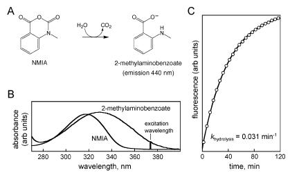
*Figure 3.* NMIA hydrolysis. (A) Reaction of NMIA with water to form the fluorescent 2-methylaminobenzoate. (B) Formation of the 2-methylaminobenzoate product is accompanied by a shift in absorbance maximum from 320 to 335 nm; product fluorescence was thus detected by exciting at 375 nm (heavy line) to eliminate inner filter effects. (C) Pseudo-first-order hydrolysis of NMIA (25 °C); every tenth data point is shown.
