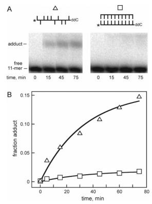
**Figure 6.** 2'-Hydroxyl acylation by NMIA is selective for unpaired nucleotides. (A) 2'-Adduct formation with the oligonucleotide (5'-UAC-UAACACC-ddC) and the corresponding duplex visualized by gel electrophoresis. Site of [32P]-label is indicated with an asterisk. (B) Quantitative analysis of 2'-O-adduct formation averaged over the 10 hydroxyl groups in the labeled oligonucleotide. Rates for the single strand (triangles) and duplex (squares) were obtained by fitting to eq 1.
