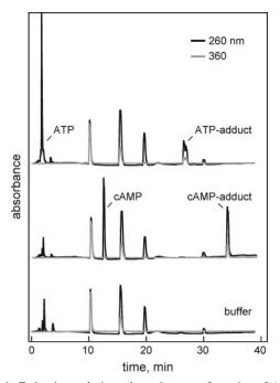
**Figure 4.** End point analysis to determine rate of reaction of ATP and cAMP with NMIA. Reaction endpoints were quantified by HPLC. Fraction ATP or cAMP product was obtained by integration of the indicated peaks. Assignment of nucleotide starting material, products, and buffer components is straightforward because all components absorb at 260 nm, whereas only 2-methylaminobenzoate products are detected at 360 nm.
