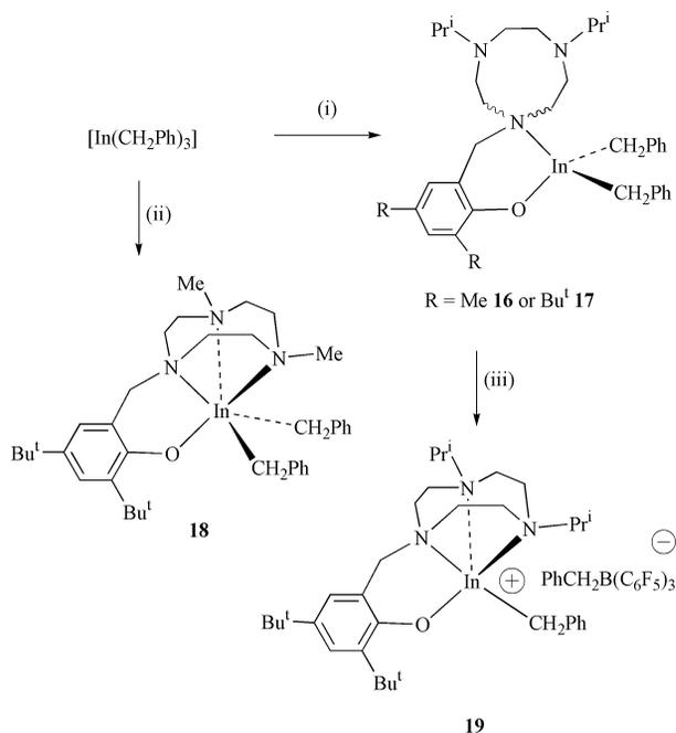
**Scheme 3** Reagents and conditions: (i)  $\text{HL}^1$  or  $\text{HL}^2$ , benzene, rt, 24 h, 73 (**16**) or 71% (**17**); (ii)  $\text{HL}^3$ , benzene, 16 h, 78%; (iii)  $\text{B}(\text{C}_6\text{F}_5)_3$ , benzene, rt, 3 h, 78%.
