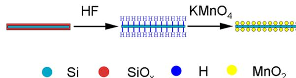
FIG. 1. (Color online) Schematic for the fabrication of MnO<sub>2</sub>/SiNWs.
