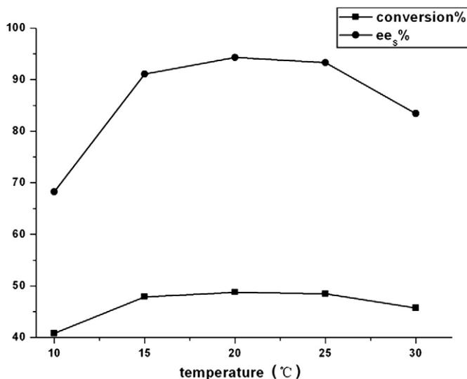
**Fig. 4.** Effect of reaction temperature on the enzymatic acylation conversion and ee<sub>s</sub> of 2-HA. Reaction conditions, varying temperature from 10 °C to 30 °C; Methyl methoxyacetate, 4 mmol; 2-HA: 5 mmol; Novozyme435: 200 mg; 10 ml ethyl ether was used as solvent.
