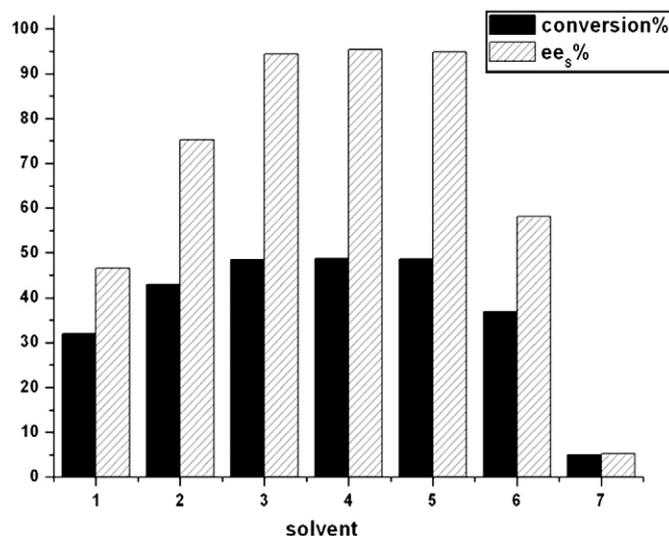
Fig. 2. Effect of solvent on the enzymatic acylation conversion and  $ee_s$  of 2-HA. Reaction conditions: methyl methoxyacetate, 4 mmol; 2-HA: 5 mmol; Novozyme435: 200 mg; solvent (10 ml): 1 n-heptane, 2 n-hexane, 3 isopropyl ether, 4 methyl tert-butyl ether, 5 ethyl ether, 6 THF, and 7 isopropanol; a slightly elevated temperature 20 °C was used during the reactions.
