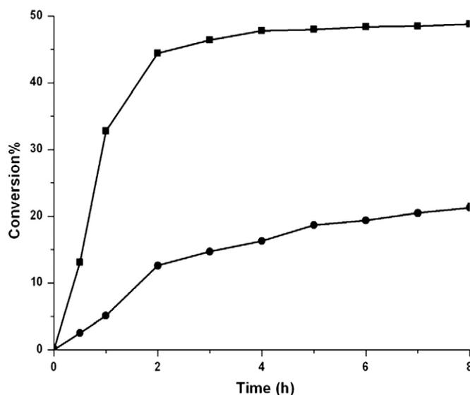
Fig. 3. Effect of acyl donor on the enzymatic acylation conversion of 2-HA. Reaction conditions: (■) methyl methoxyacetate, 4 mmol (●) methyl dimethoxyacetate, 4 mmol; 2-HA: 5 mmol; Novozyme435: 200 mg; 10 ml ethyl ether was used as solvent. A slightly elevated temperature 20 °C was used during the reaction.
