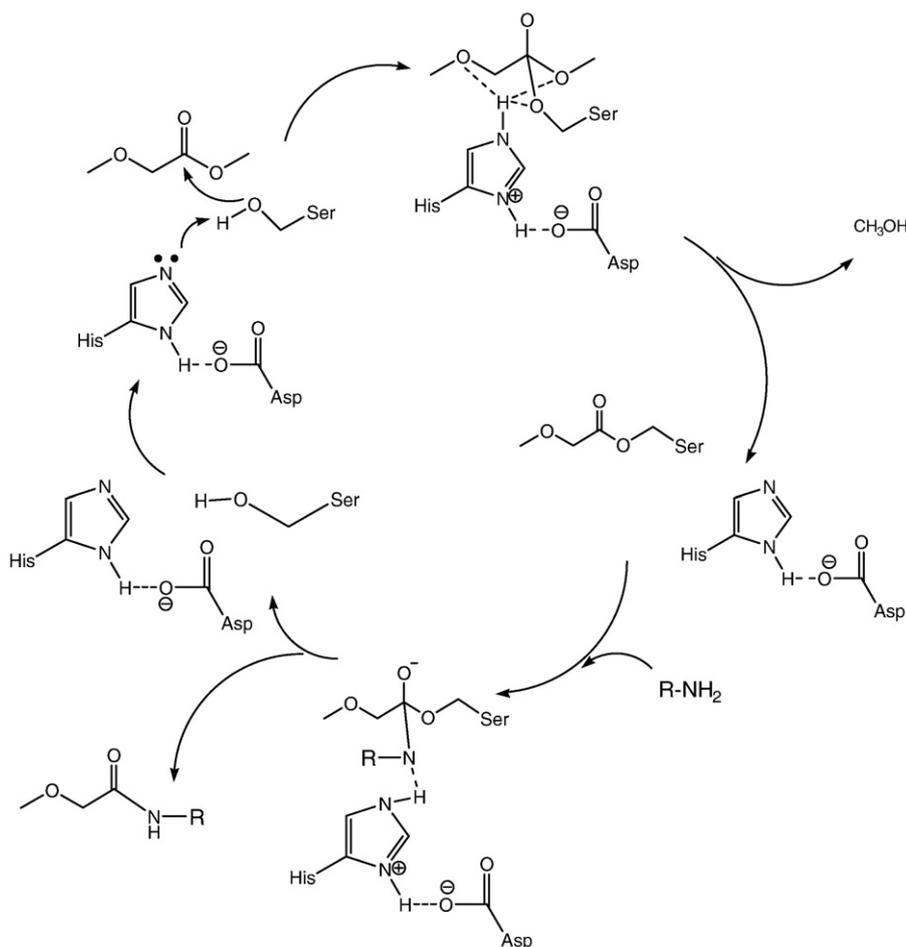
**Scheme 2.** Enzymatic kinetic acylation mechanism of amines.
