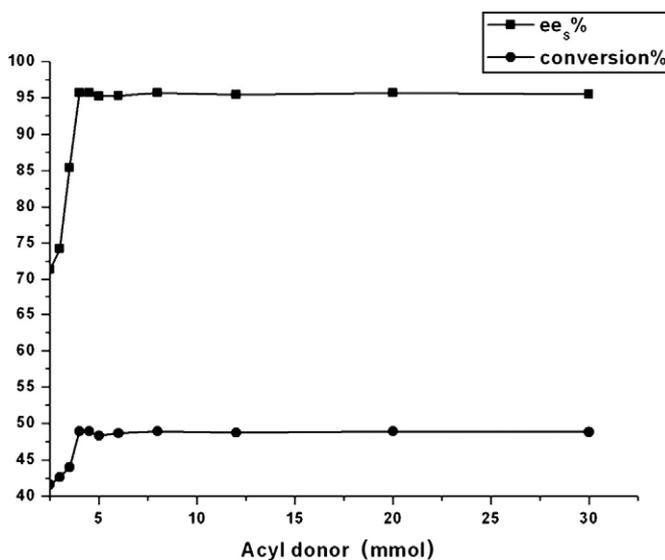
**Fig. 5.** Effect of amount of acyl donor on the enzymatic acylation conversion and ee<sub>s</sub> of 2-HA. Reaction conditions, varying the amount of methyl methoxyacetate from 2.5 mmol to 30 mmol; 2-HA: 5 mmol; Novozyme435: 200 mg; 10 ml ethyl ether was used as solvent. A slightly elevated temperature 20 °C was used during the reaction.
