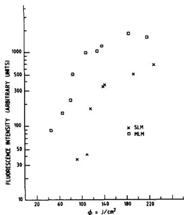
Figure 2: Integrated Fluorescence Intensity vs  $CO_2$  Laser Fluence for different pulse intensities under collisionless conditions.
