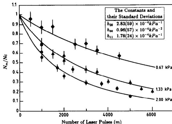
Figure 3: Fraction of  $CDCl_3$  remaining versus number of pulses for various initial pressures of  $CDCl_3$ . The initial pressures in kPa are represented by a,  $\blacklozenge$  for 0.67,  $\blacktriangle$  for 1.33 and  $\bullet$  for 2.00 respectively.
