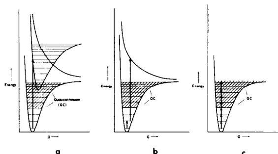
Figure 1: a. Selective, one-photon predissociation process; b. Selective two-step, two-photon, process; c. Selective MPD process
