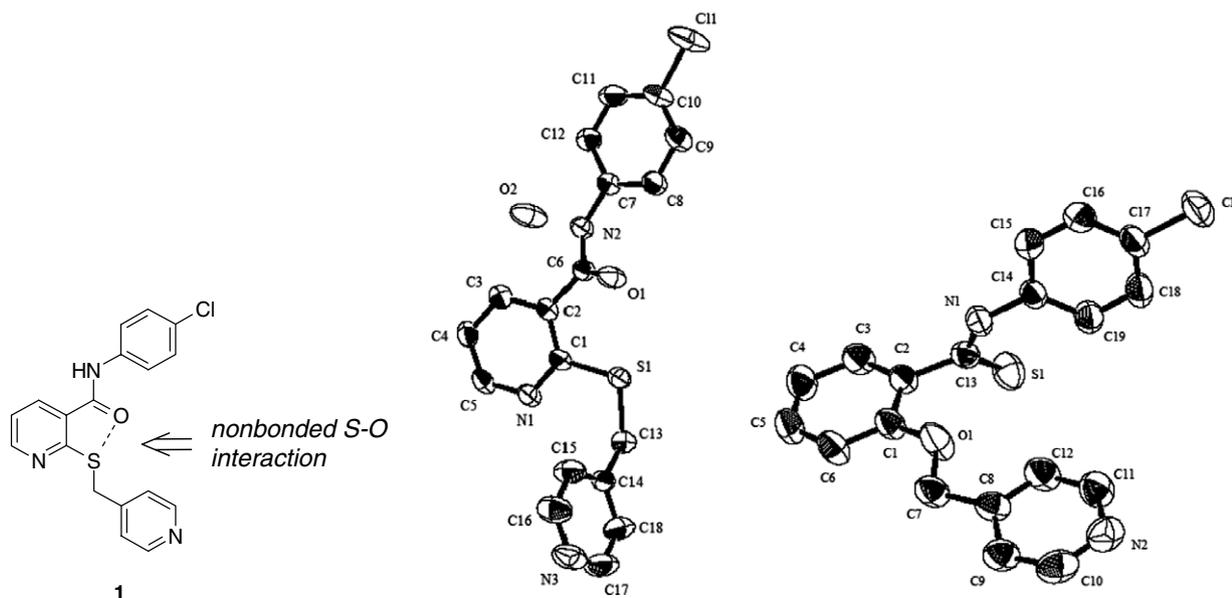
Figure 5. Left, structure of compound **1**; middle, ORTEP drawing of compound **1** (monohydrate) (S–O; 2.82 Å,  $\chi = 35^\circ$ ); right, ORTEP drawing of compound **9** (S–O; 3.79 Å,  $\chi = 108^\circ$ ).
