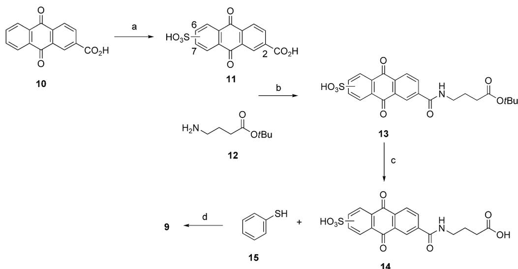
Scheme 3. Synthesis of anthraquinone-tethered acyl donor **9**. a) 30%  $\text{SO}_3/\text{H}_2\text{SO}_4$ , microwave (300 W), 170 °C, 15 min, 90%; b) DMT-MM, NEM, MeOH/ $\text{H}_2\text{O}$  3:1, RT, 19 h, 94%; c) TFA,  $\text{CH}_2\text{Cl}_2$ , RT, 3 h, 100%; d) DMT-MM, NEM, MeCN, RT, 5 h, 40%. TFA = trifluoroacetic acid.
