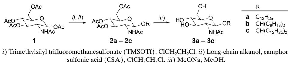
i) Trimethylsilyl trifluoromethanesulfonate (TMSOTf), ClCH<sub>2</sub>CH<sub>2</sub>Cl. ii) Long-chain alcohol, camphor-sulfonic acid (CSA), ClCH<sub>2</sub>CH<sub>2</sub>Cl. iii) MeONa, MeOH.
