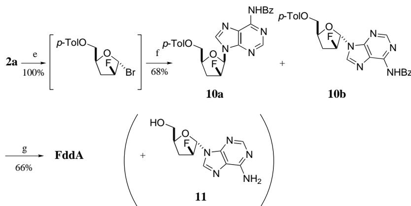
**Scheme 2.** Reagents and conditions: (e) AcOH–HBr, CH<sub>2</sub>Cl<sub>2</sub>; (f) *N*-benzoylaminopurine, NaH, THF, reflux; (g) MeONa, MeOH, reflux.
