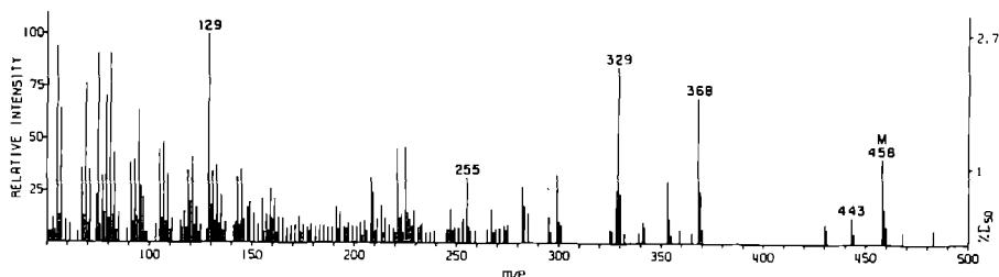
Figure 3. Mass spectrum of the TMS ether of unknown 1 (peak 1 in fig. 1).
