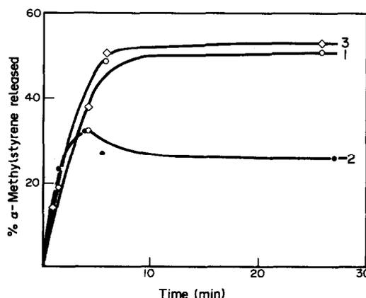
Fig. 3. Kinetic curves of reaction (5), as followed by measuring the liberation of  $\alpha$ -methylstyrene from **VIb** by GLC: 1—LiCl, 2—LiBr and 3—LiI; 80°C, HOAc— $\text{CHCl}_3$ .
