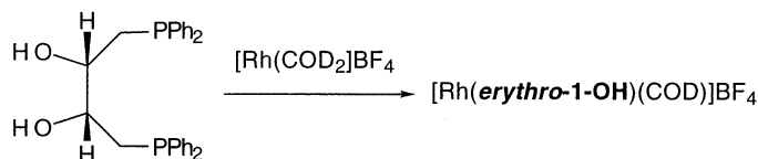
Scheme 3. Synthesis of [\text{Rh}(\text{erythro-1-OH})(\text{COD})]\text{BF}_4 .
