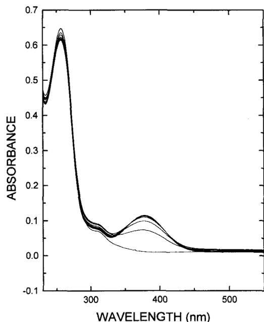
**Figure 2.** Absorption spectra of the reduced form of NAD<sup>+</sup> analog 1 at 1 h intervals. The NAD<sup>+</sup> analog 1 was converted to its reduced form by incubating with equine LADH with ethanol as substrate at room temperature for 12 h. The substrate concentration used was 0.2 M ethanol and 37  $\mu$ M NAD<sup>+</sup> analog 1 in 65 mM Trizman buffer (pH 8.8).
