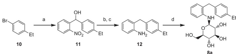
Scheme 1. Synthesis of aniline-N-glucosides **8a**. Reagents and conditions: (a) *n*-BuLi, THF, −78 °C, then *o*-nitrobenzaldehyde, THF, −78 to 0 °C (27%); (b) H<sub>2</sub>, Pd/C, EtOH, rt (100%); (c) Et<sub>3</sub>SiH, BF<sub>3</sub>·Et<sub>2</sub>O, MeCN, −78 °C to rt (75%); (d) *D*-(+)-glucose, NH<sub>4</sub>Cl, MeOH, reflux (56%).
