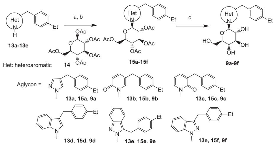
**Scheme 2.** Synthesis of heteroaromatic-N-glucosides **9a–9f**. Reagents and conditions: (a) *N,O*-bis(trimethylsilyl)acetamide, MeCN, 60 °C; (b) **14**, trimethylsilyl triflate, 1,2-dichloroethane, 80 °C (**15a** 44%, **15b** 37%, **15c** 4%, **15d** 17%, two steps); (c) NaOMe, MeOH, rt (**9a** 78%, **9b** 82%, **9c** 48%, **9d** 48%) (**9e** 42% and **9f** 5% based on **13e**, respectively).
