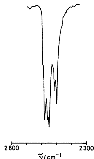
FIGURE 3 \nu(\text{B-H}) region of the solid-state i.r. spectrum of cis - [\text{Pt}(\text{B}_5\text{H}_8)\text{Cl}(\text{dppe})] (KBr disc) exhibiting strong peaks at 2580 , 2560 , 2550 , 2520 , and 2500\text{ cm}^{-1} . The spectrum of a solution in \text{CH}_2\text{Cl}_2 shows loss of fine structure to give two broader peaks with \nu_{\text{max}} at 2560 and 2520\text{ cm}^{-1}
