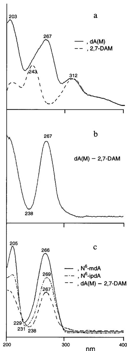
**Figure 3.** UV spectra and computed UV difference spectra of the MC–deoxyadenosine adduct **8**, 2,7-DAM, and deoxyadenosine. Comparison with standard  $N^6$ -alkyldeoxyadenosines: (a) UV spectra of dA(M) (adduct **8**) and 2,7-DAM (**6**), (b) difference spectrum of dA(M) – 2,7-DAM (**8** – **6**), (c) spectra of  $N^6$ -mdA,  $N^6$ -ipdA, and their comparison with the difference spectrum of dA(M) – 2,7-DAM in panel b.
