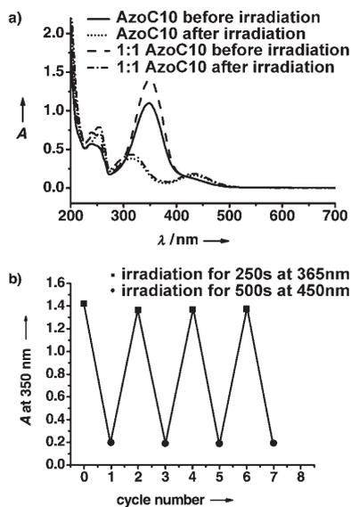
**Figure 3.** a) Photoisomerization spectra of AzoC10 in the presence of  $\alpha\text{-CD}$  (1:1 molar ratio) before and after UV irradiation. b) Changes of AzoC10–CD inclusion (absorbance at 350 nm) upon alternating irradiation with UV and visible light. The concentration of AzoC10 is  $7 \times 10^{-5} \text{ M}$ .
