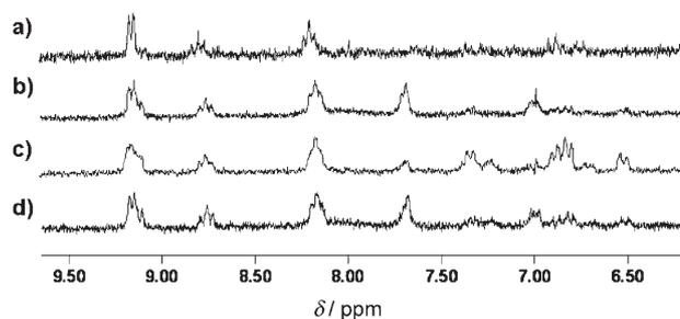
**Figure 5.** <sup>1</sup>H NMR spectra of a) AzoC10, b) AzoC10 in the presence of  $\alpha$ -CD (1:1 molar ratio), and c) after irradiation at 365 nm for 500 s, then d) irradiation at 450 nm for 2700 s. The concentration of AzoC10 is 2.5 × 10<sup>-4</sup> M. The solvent is D<sub>2</sub>O;  $\delta(\text{H}_2\text{O}) = 4.79$  ppm.
