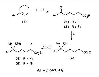
Scheme 1. Reagents: i, O<sub>3</sub>, CH<sub>2</sub>Cl<sub>2</sub>; Me<sub>2</sub>S, -78 °C; ii, Jones oxidation, acetone; iii, EtOH, H<sub>2</sub>SO<sub>4</sub>, reflux; iv, MeLi, benzene, 0 °C; v, PhSH, ZnI<sub>2</sub>, ClCH<sub>2</sub>CH<sub>2</sub>Cl, room temp.; vi, LiNPri<sub>2</sub>, tetrahydrofuran (THF), HCO<sub>2</sub>Et, -78 °C; vii, *p*-MeC<sub>6</sub>H<sub>4</sub>-SO<sub>2</sub>N<sub>3</sub>, Et<sub>3</sub>N, CH<sub>2</sub>Cl<sub>2</sub>, room temp.
