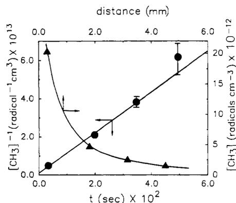
**Figure 1.** Plots of  $[CH_3^*]$  versus probe distance and  $[CH_3^*]^{-1}$  versus time (time for gas flow from catalyst bed to the probe).
