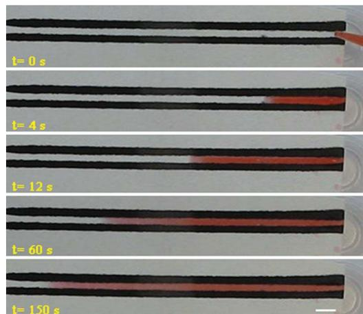
**Fig. 4** Sequence of video frames from a  $\mu$ PAD formed on Whatman grade 1 paper tracking the movement of 20  $\mu$ L of a red food dye solution. Stamping conditions: PDMS stamp border width 1100  $\mu$ m, Black Lumocolor<sup>®</sup> ink thinned formulation, average flow speed = 1.3 mm s<sup>-1</sup> (scale bar: 3.5 mm).
