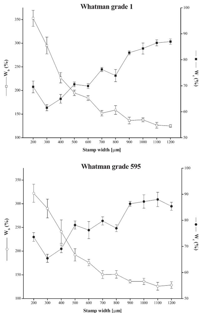
**Fig. 3** Percentage of border width variation ( $W_b$ ) and final channel width ( $W_c$ ) for open straight channels with different border width on Whatman grade 1 (top) and grade 595 (bottom) filter papers ( $n = 5$ ).
