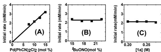
**Figure 1.** The dependence of the initial rate on: (A) [Pd(PhCN)<sub>2</sub>Cl<sub>2</sub>] (1<sup>st</sup>-order), (B) [<sup>t</sup>BuONO] (0<sup>th</sup>-order), and (C) [**1a**]: (0<sup>th</sup>-order). For details, see SI.
