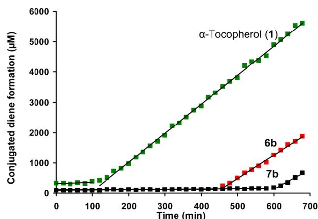
**Figure 2.** Peroxidation traces (conjugated diene formation vs time) recorded using compounds **1**, **6b**, and **7b** ( $40\text{ }\mu\text{M}$ ) as antioxidants in the chlorobenzene layer in the presence of NAC (1 mM) in the aqueous phase.
