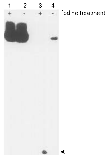
Figure 7. Autoradiogram of a 20% denaturing polyacrylamide gel demonstrating the topoisomerase I-mediated formation of the bridging phosphorothioate linkage. Lane 1, I 2 treatment of the product resulting from ligation of I with the topoisomerase I–DNA covalent complex; lane 2, product resulting from ligation of I with the topoisomerase I–DNA covalent complex; lane 3, I 2 treatment of the product resulting from ligation of III with the topoisomerase I–DNA covalent complex; lane 4, product resulting from ligation of III with the topoisomerase I–DNA covalent complex.
