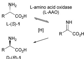
**Scheme 1** Deracemisation of an  $\alpha$ -amino acid D/L-1 using a combination of an L-amino acid oxidase (L-AAO) and reducing agent.
