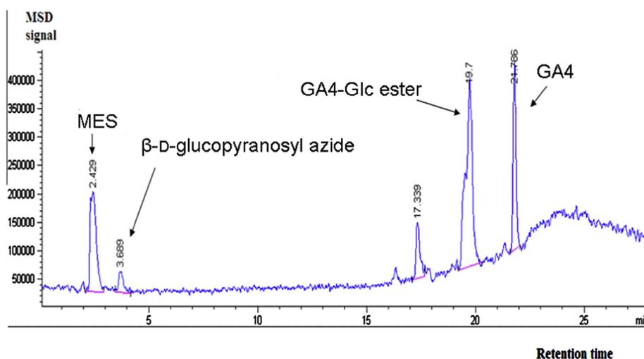
**Fig. 1.** The LC-MS chromatogram of the transglycosylation reaction of Os3BGlu6 E178A with GA<sub>4</sub>-GE as donor and sodium azide as acceptor. The reaction components were separated by C18 reverse phase HPLC, as described in the methods. The detector was an Agilent MSD single quadrupole mass spectrometer with API-ES source in negative ion mode, with a scan range of 50–800 m/z.
