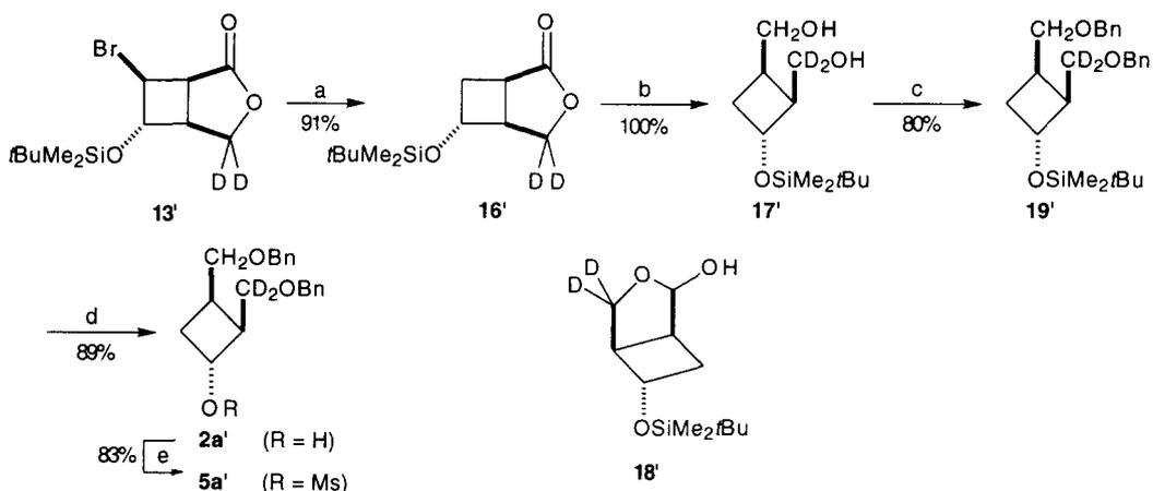
(a) *n*-Bu<sub>3</sub>SnH, AIBN, Toluene, 7h, r.t.; (b) LiAlH<sub>4</sub> (5 eq), THF, 4h, r.t.; (c) NaH, PhCH<sub>2</sub>Br, DMF, 5h, r.t.; (d) *n*-Bu<sub>4</sub>NF, THF, 23h, r.t.; (e) MsCl, Et<sub>3</sub>N, CH<sub>2</sub>Cl<sub>2</sub>, 0°C, 1h 30min.
