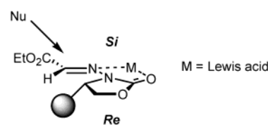
FIGURE 1. A model explaining the stereochemical outcome of the Mannich-type reactions with hydrazones 3a–c .
