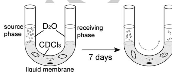
**Figure 7.** An apparatus for hexose transport through a membrane filter.
