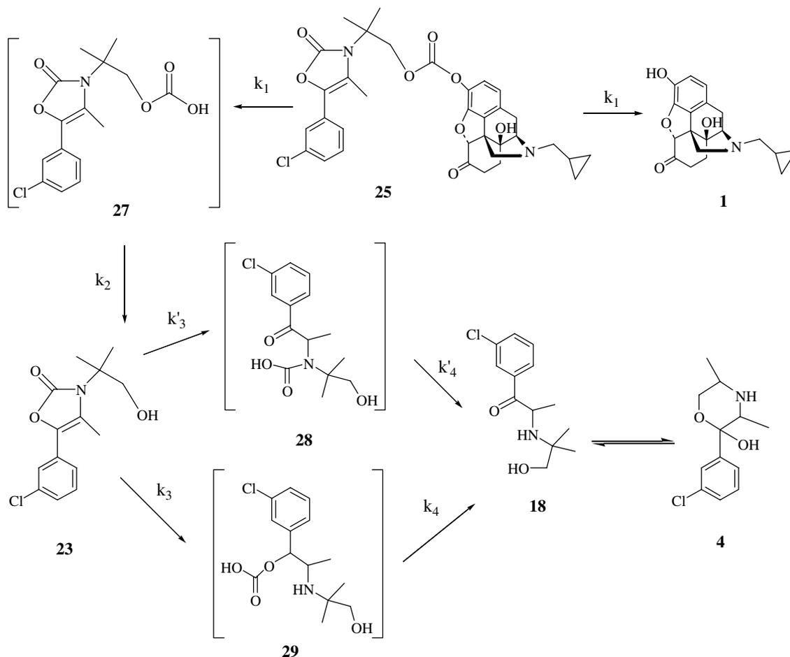
**Scheme 4.** A schematic diagram showing stepwise hydrolytic cleavage of the carbonate codrug **25** into NTX and BUPOH in isotonic phosphate buffer, pH 7.4.
