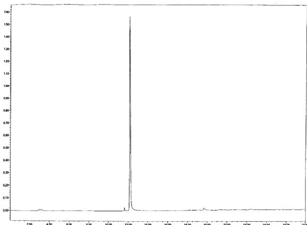
**Fig. 1** HPLC profile of the compound **9**. Conditions: COSMOSIL 5C18-MS column (4.6 × 250 mm); eluent A, 0.1% TFA/water; eluent B, 0.1% TFA/acetonitrile; gradient, linear 0–100% B over 35 min; detection 260 nm; flow rate, 1 mL/min; 55 °C.
