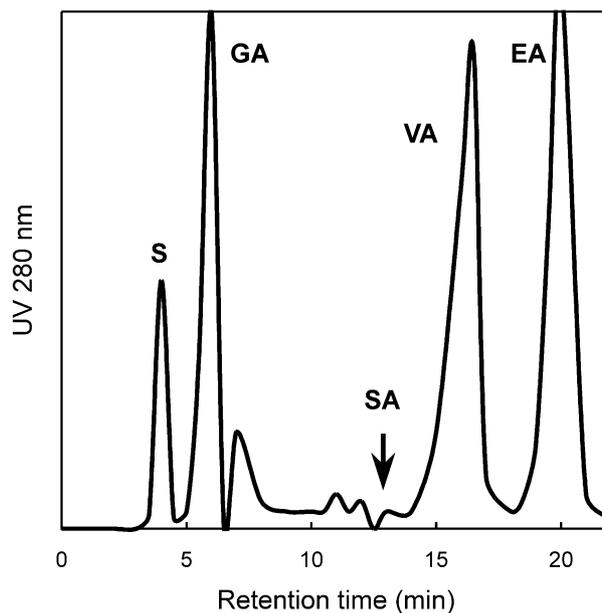
Fig. 3. HPLC analysis of phenolic components after total acid hydrolysis of the enzyme reaction product, cornusiiin E (3). S, Solvent peak; GA, gallic acid; VA, (*S*)-valoneic acid; EA, ellagic acid. The retention time of (*S*)-sanguisorbic acid (SA), a naturally occurring isomer of valoneic acid with the galloyl residue attached in *ortho*-position to the HHDP moiety, is indicated by the arrow.
