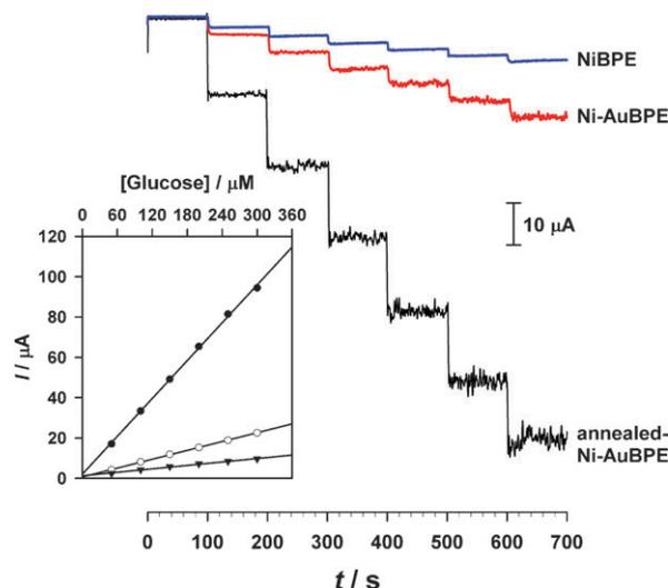
**Fig. 4** The chronoamperometric experiments of the stepwise addition of  $50 \mu\text{M}$  glucose at NiBPE, Ni–AuBPE and annealed Ni–AuBPE in  $0.1 \text{ M NaOH}$ . The inset shows linear calibration plots obtained at NiBPE ( $\blacktriangledown$ ), Ni–AuBPE ( $\circ$ ) and annealed Ni–AuBPE ( $\bullet$ ), respectively.
