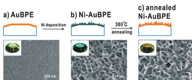
**Fig. 1** Schematic of the fabrication process and the SEM images of (a) AuBPE, (b) Ni–AuBPE and (c) annealed Ni–AuBPE, respectively.
