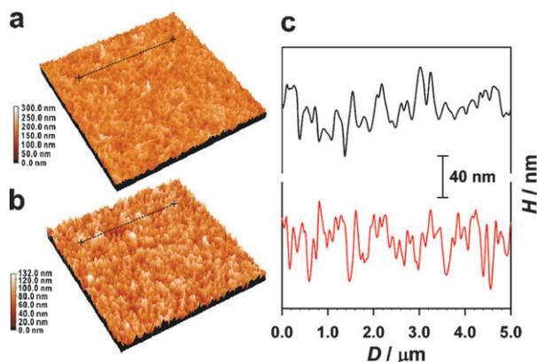
**Fig. 2** AFM images of (a) Ni–AuBPE and (b) annealed Ni–AuBPE, respectively. (c) The surface outlines of Ni–AuBPE (black line) and annealed Ni–AuBPE (red line).
