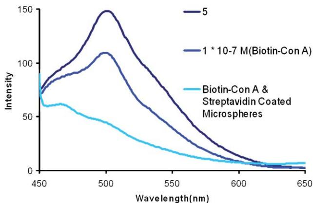
**Fig. 3** Fluorescence of aggregates of **5** and biotinylated ConA before and after addition of streptavidin-coated microspheres.
