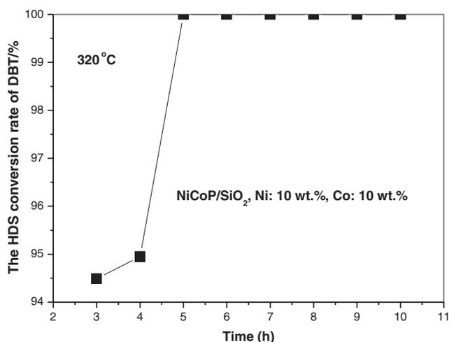
**FIGURE 5** The HDS activity for DBT of the NiCoP/SiO<sub>2</sub> (Ni: 10 wt.%, Co: 10 wt.%) obtained at 700 °C for 15 min
