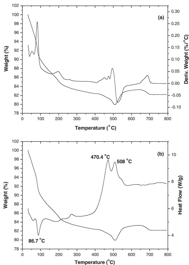
**FIGURE 3** TG/DTG analysis of the NiCoP/SiO<sub>2</sub> (Ni: 10 wt.%, Co: 10 wt.%) obtained at  $700\text{ }^{\circ}\text{C}$  for 15 min
