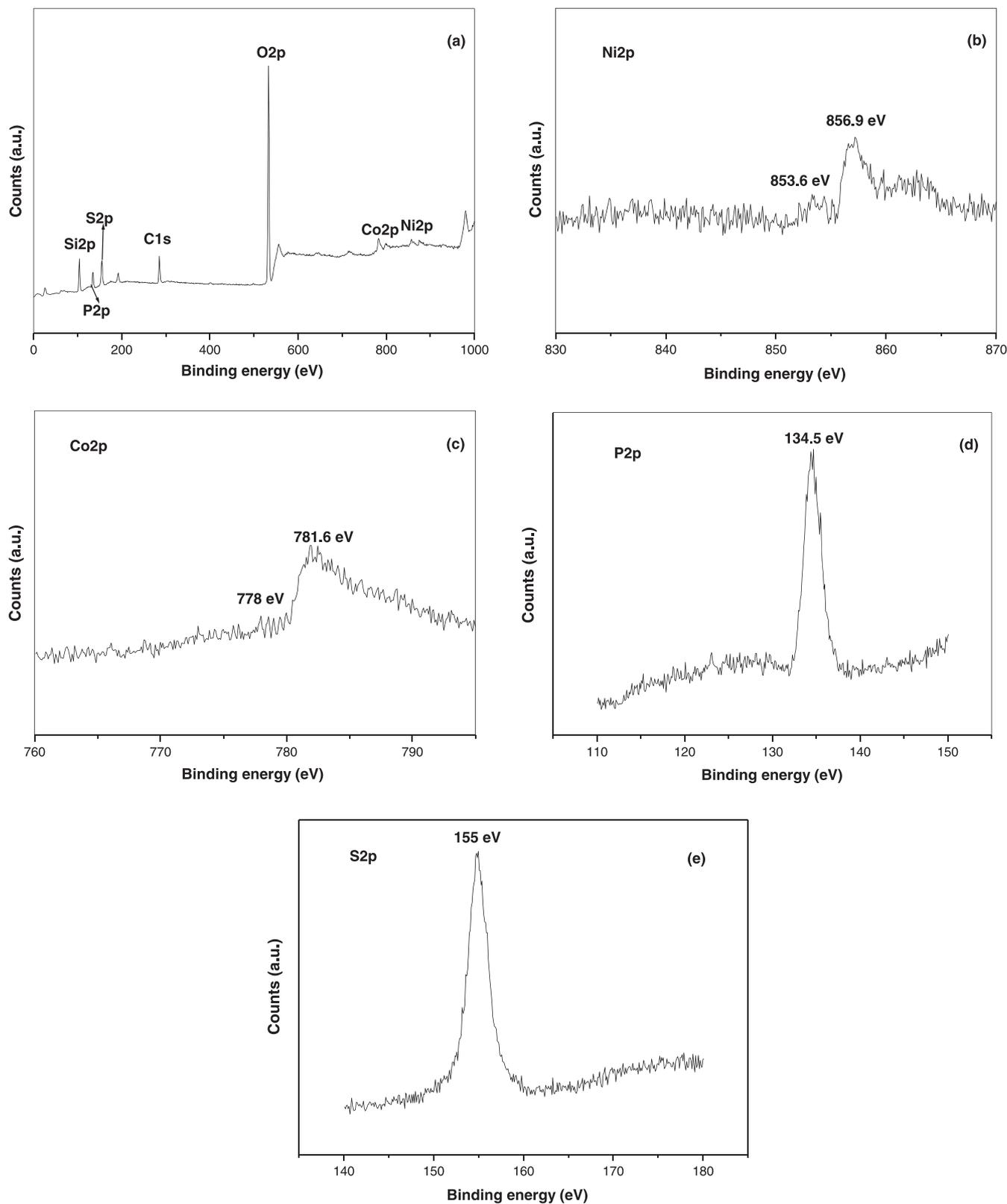
**FIGURE 4** XPS spectra of the NiCoP/SiO<sub>2</sub> (Ni: 10 wt.%, Co: 10 wt.%) obtained at 700 °C for 15 min. (a) Survey, (b) Ni2p, (c) Co2p, (d) P2p, (e) S2p
