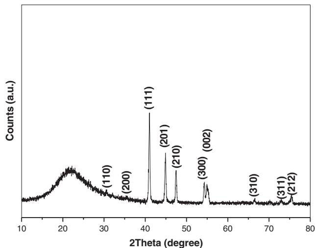
**FIGURE 1** X-ray diffraction patterns of NiCoP/SiO<sub>2</sub> (Ni: 10 wt.%, Co: 10 wt.%) obtained at 700 °C for 15 min
