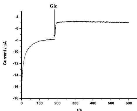
**Fig. 7** A typical biosensor response to glucose (in 50 mM sodium acetate buffer, pH 5.5; 25 °C;  $-0.7$  V, [Glc]; 0.75 mM).
