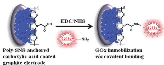
**Scheme 1** A schematic representation of the construction of the proposed glucose biosensor.
