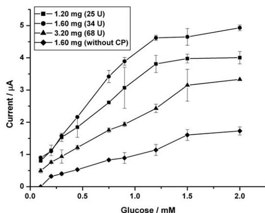
**Fig. 2** Effect of loaded enzyme amount (in sodium acetate buffer, 50 mM, pH 5.5; 25 °C). Error bars show standard deviation (SD) of three measurements for each.
