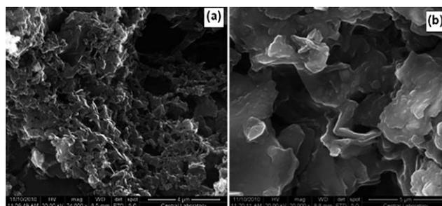
**Fig. 3** SEM images of polymer before (a) and after biomolecule immobilization (b) under optimized conditions. Magnification (a) 24000; (b) 20000.
