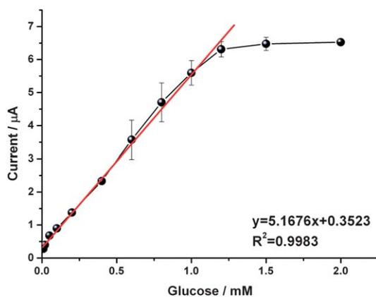
**Fig. 6** Calibration curve for glucose (in 50 mM sodium acetate buffer, pH 5.5; 25 °C;  $-0.7$  V). Error bars show standard deviation (SD) of three measurements for each.
