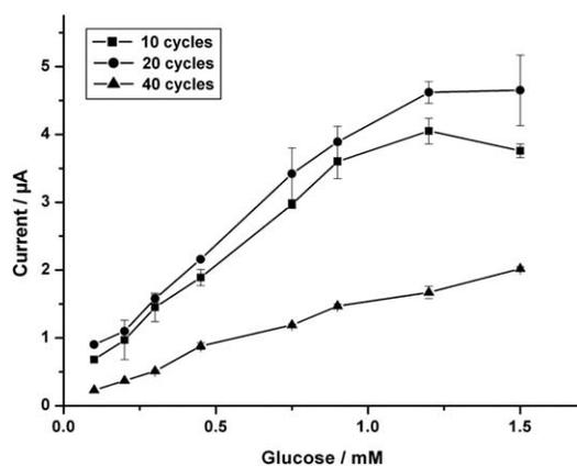
**Fig. 4** Effect of polymer layer thickness (in sodium acetate buffer, 50 mM, pH 5.5; 25 °C). Error bars show standard deviation (SD) of three measurements for each.
